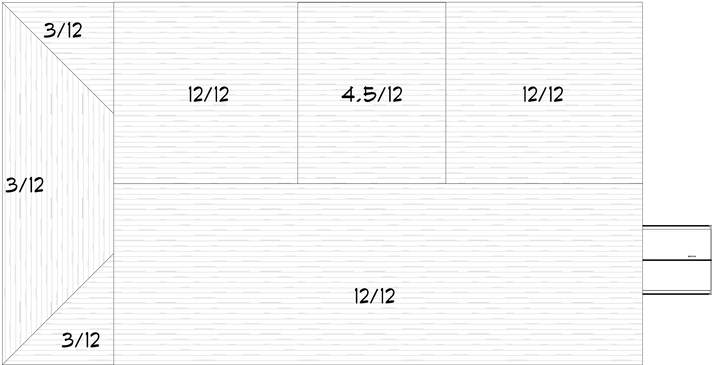
ROOF VIEW SCALE: 1/4" = 1'-0"
